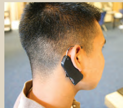
↑ The postural assist device senses when a blind person’s head is in an undesirable position – such as slouched or tilted to the side – and alerts them.
