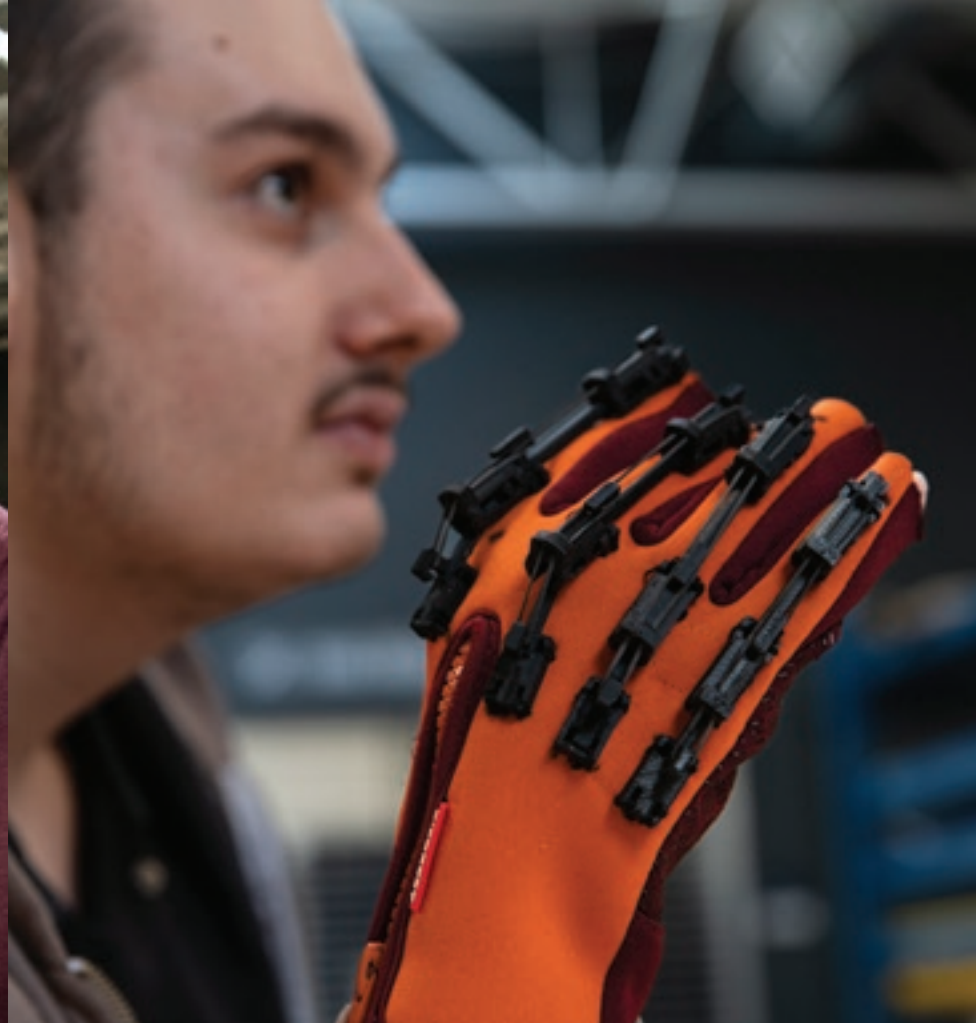
Above: The "gauntlet" is a synthetic fiber glove married to a tension-assisting exoskeleton that strengthens Brandon's finger movements.
